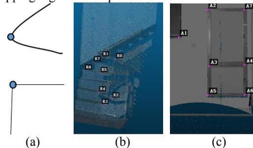
**Fig.2.** (a) ordinary corner feature, (b) and (c) are the different corner features extracted from point cloud sets
