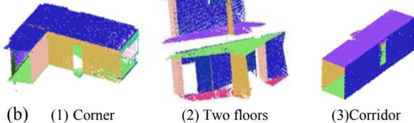
**Fig.3** (a)The illustration of deciding plane points, (b)Plane extraction works well in different indoor structures with our testing environment
