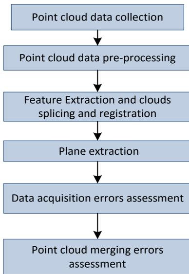
**Fig.1.** The procedure quality evaluation Framework for Point Cloud model
