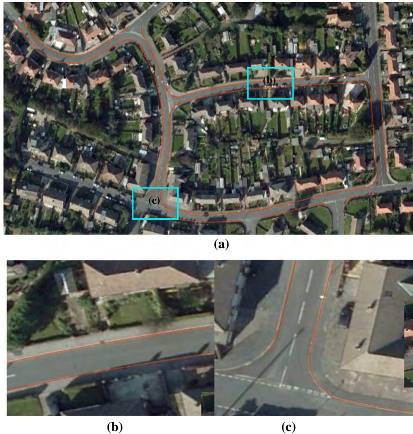
Fig. 17. Registration of extracted curb points and the Google Earth image (residential area).
