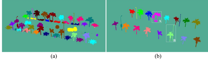
Fig. 5. (a) Clustering result using the Euclidean distance clustering approach. (b) Filtering result using prior knowledge.
