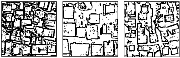
Figure 5. Binary images of the extracted edges of shack roofs with noise.
