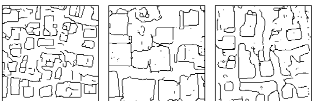
Figure 7. Shack roof outlines delineated after thinning.
