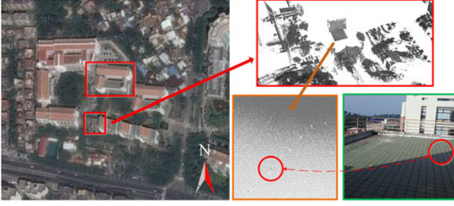
Fig. 8. Experimental dataset: image on the left showing the geographical position of survey scenes; image on the right an illustration of data collection procedure (the red box shows the scanning point clouds, the green box the targets placement in scene, and the orange box the same targets scanned into point clouds).
