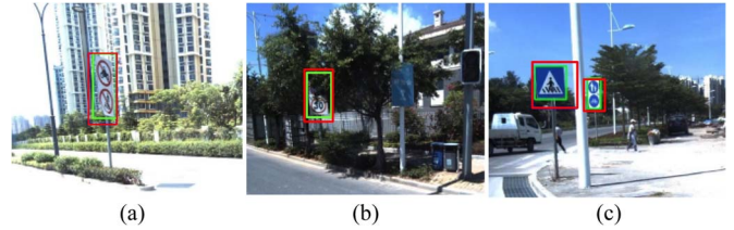
Fig. 12. Examples of traffic sign detected in challenging scenarios. (a) strong illumination and large viewpoint, (b) partial occlusions, (c) cluttered background.
