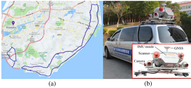
Fig. 3. Roads and system for MLS data acquisition: (a) trajectory (in blue color) in Xiamen Island for data acquisition, (b) MLS system used.
