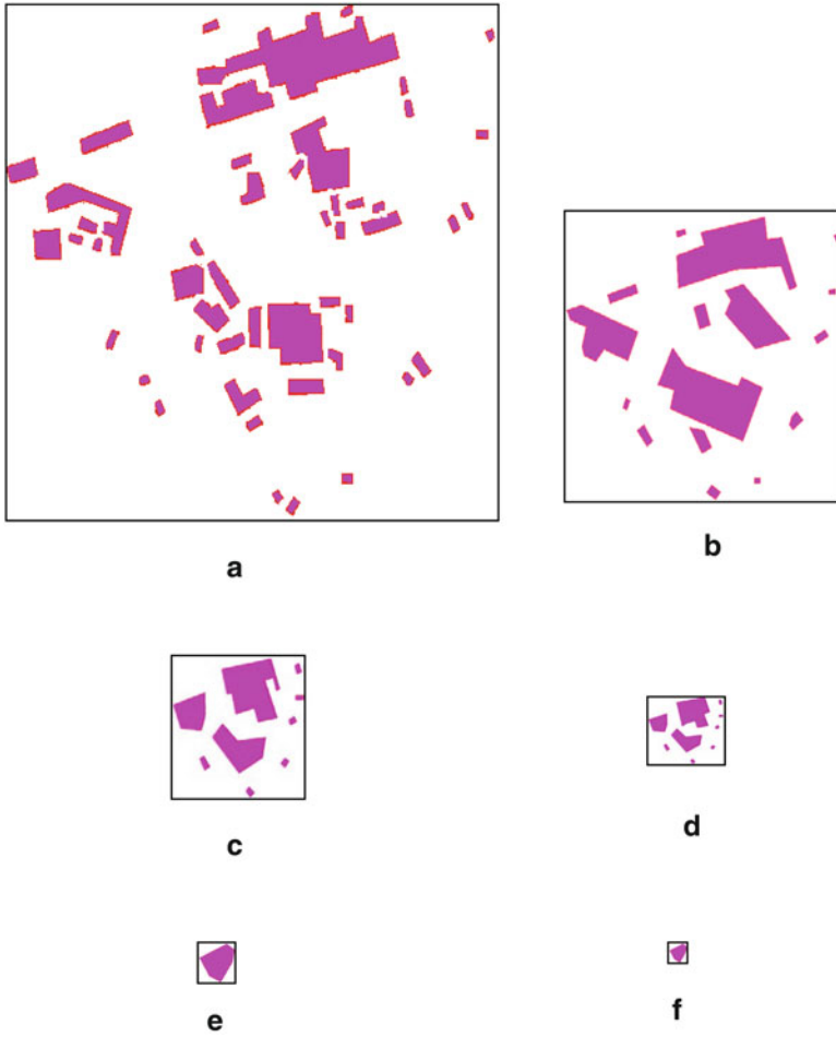
Fig. 5.26 Experiment 26: complex settlements at different map scales. The settlements are complex shaped but basically orthogonal in the corners and show different orientations and little parallelism. (a) 1:10 K; (b) 1:25 K; (c) 1:50 K; (d) 1:100 K; (e) 1:250 K; and (f) 1:500 K
