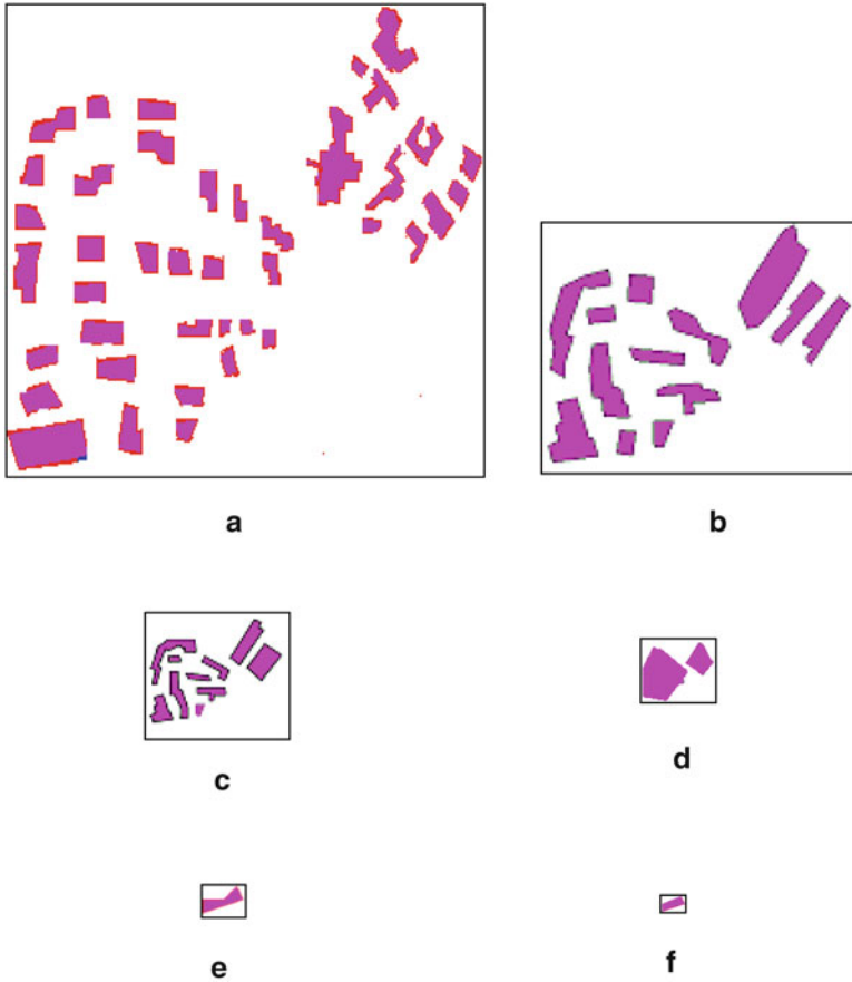
Fig. 5.27 Experiment 27: irregular-shaped settlements at different map scales. The settlements have complex and nonconvex shapes with arbitrary angles in the corners and have arbitrary orientations and little parallelism. (a) 1:10 K; (b) 1:25 K; (c) 1:50 K; (d) 1:100 K; (e) 1:250 K; and (f) 1:500 K
