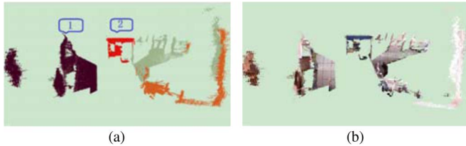
Fig. 8. Nonoverlapping frame alignment. (a) Two local data frames required. (b) Aligning nonoverlapping frames by robot pose.
