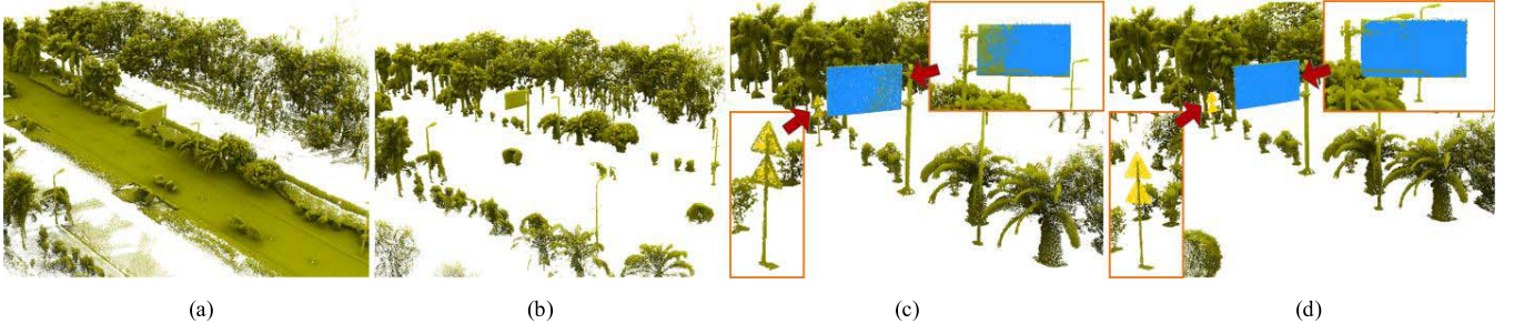
Fig. 3. The process of traffic sign detection: (a) raw point clouds, (b) ground removal, (c) traffic sign detection results, (d) the repaired results after region growth.
