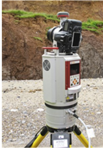
Figure 1. Our 3D Scanning System. The top part is camera and the bottom part is laser scanner.
