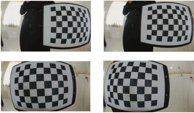
Fig. 3. Sample of the images for the fisheye camera calibration.
