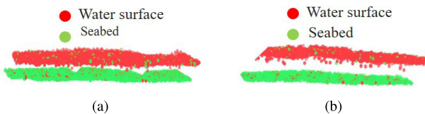
Fig. 8. Classified semantic labels of water surface and seabed in different water depth via SPG with VSP. (a) Shows the semantic label with depth of 0.8 to 1.5 m in shoreline. (b) Shows the semantic label with depth of more than 2.5 m.
