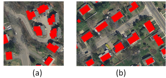
Fig. 1. Two typical errors of building footprints in OSM: (a) alignment errors between polygons (red) and real buildings and (b) shape differences between polygonal footprints and corresponding building masks.
