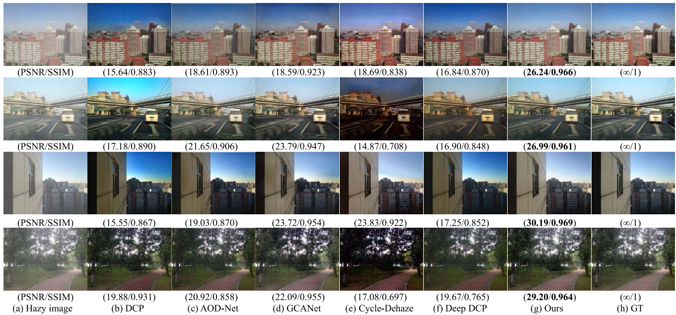
Fig. 8. Image dehazing results on the SOTS outdoor dataset. From (a) to (h): (a) the hazy image, and the dehazing results of (b) DCP [6], (c) AOD-Net [7], (d) GCANet [8], (e) Cycle-Dehaze [9], (f) Deep DCP [59], (g) our Cycle-SNSPGAN, respectively, and (h) the ground-truth image. Our Cycle-SNSPGAN can produce much clearer results with less color distortion and fewer artifacts.
