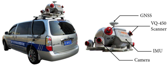
Fig. 4. Mobile laser scanning system for point clouds acquisition.
