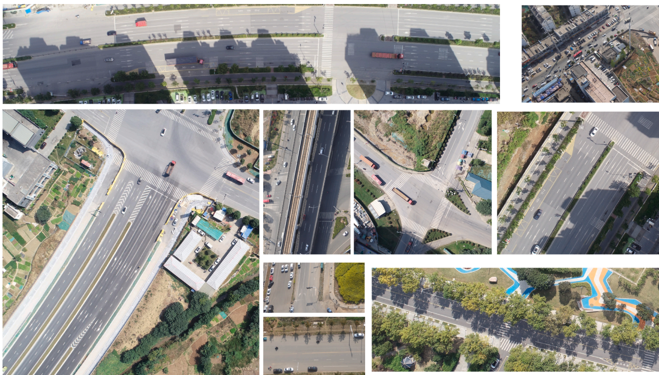
Fig. 1. Challenges in road marking segmentation. For example, shadows caused by buildings and trees; partial occlusion caused by other objects, such as vehicles; severely destroyed road markings; false road markings caused by illumination, imaging tilt angles, and other road marking materials; presence of several types of road markings with varied sizes and shapes (e.g., turn signs, pedestrian crossing, zigzag, bus and bike sign, solid and dot line lanes).
