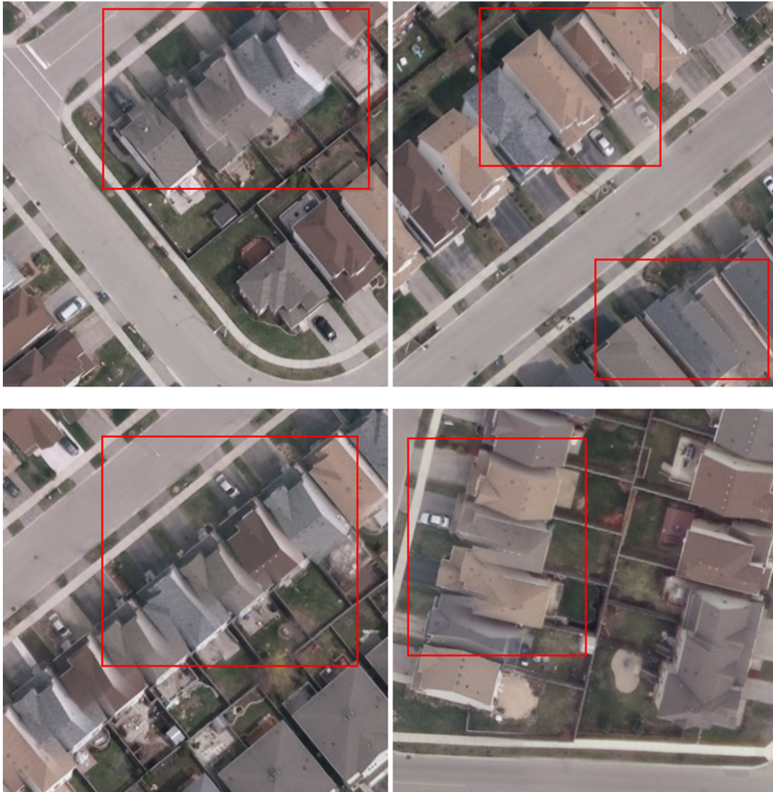
Figure 3. Examples of geometric distortion in aerial images (Tool: Microsoft Word; Data source: Waterloo building dataset (He et al. 2021)). [Colour online.]
