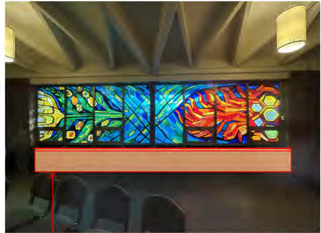
ARCH SCOPE: Veneered wood panel with solid edging up to 2' on painted steel brackets
