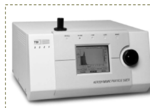
Aerodynamic Particle Sizer (APS 3321), 0.35-20 μm
