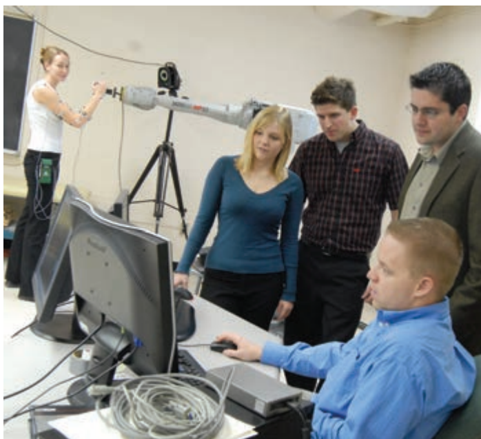
Dickerson (far right standing) and graduate students use a robotic arm and 3D motion-tracking to assess shoulder loading and posture.
