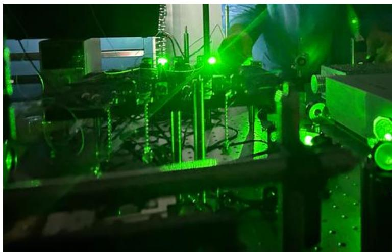
*Green laser light is the correct energy to manipulate the energy states of barium ions.*
