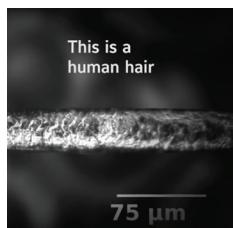
Hairs are much less than a millimeter thick, so we can't use tools like rulers to measure them. In this activity, we'll use interference to measure the width of your hair!
