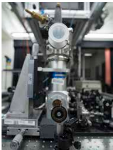
Samples are placed in this cryostat in the optics lab before a vacuum pump is used to remove the air. Liquid helium cools the chamber to about 4 Kelvin, and then lasers are used to excite the samples.
