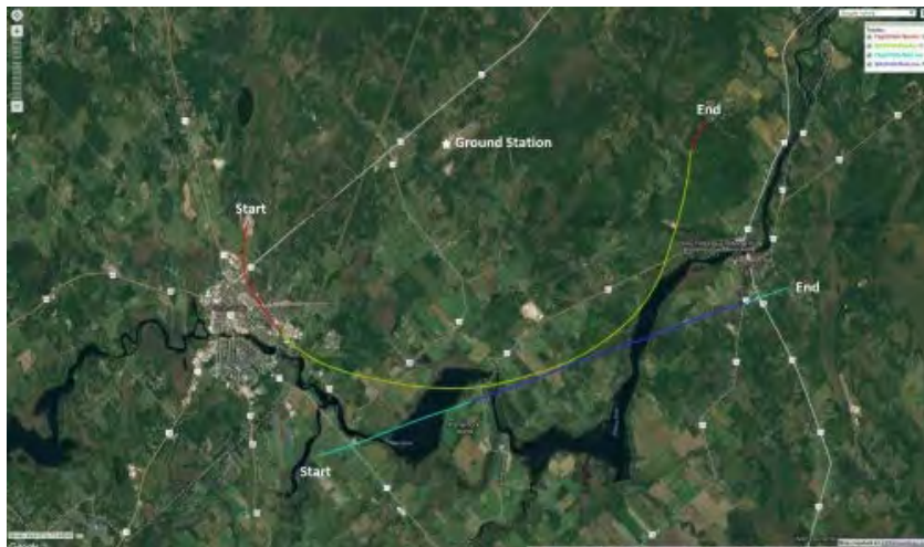
Flight paths for the 7km arc and line, followed from left to right. The star indicates the location of the ground station at Smith Falls (Montague Airport). The inner portions represent where the quantum link was active. Photo produced using GPSVisualizer.com, map data c 2016 Google, imagery c 2016 Cnes/Spot Image, DigitalGlobe, Landsat, New York GIS, USDA Farm Service Agency.
