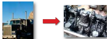
Figure 2. Sludge formation caused by circulating the exhaust gas back into the oil
