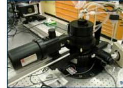
Measures the Hydrodynamic Radius ( $R_h$ ) and Radius of Gyration ( $R_g$ ) of particles in the system
