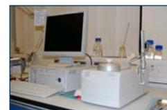
Measures the heat of binding as a titrant is added to a ligand
