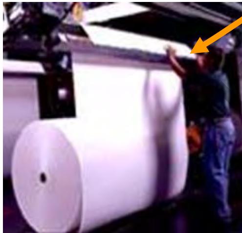
Flying-splice in papermaking mills
