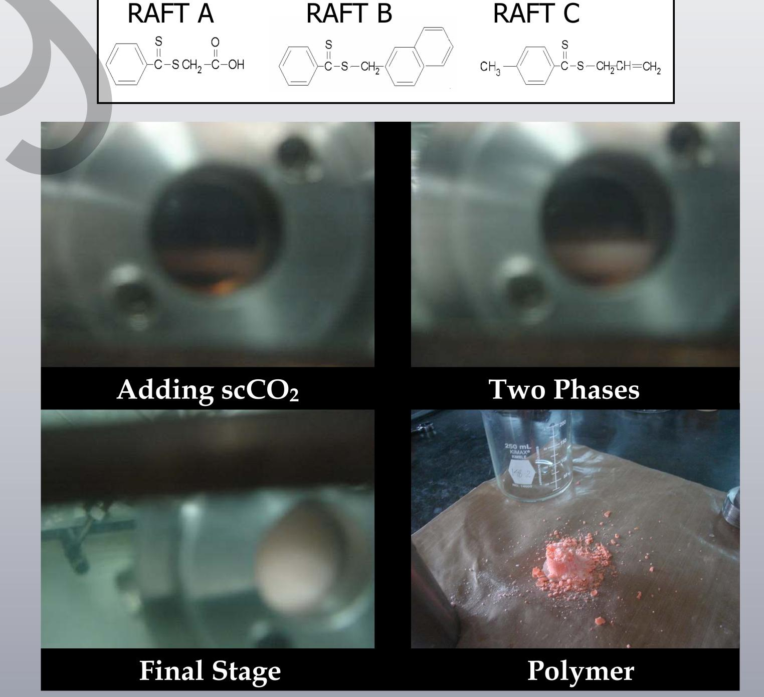
Polymerizations were carried out using AIBN as initiator and Poly(styrene-b-dimethylsiloxane), P(S-b-DMS) as surfactant.
