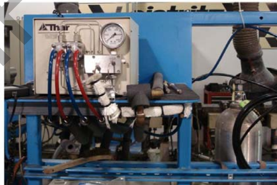
Sc Co2 injection system
