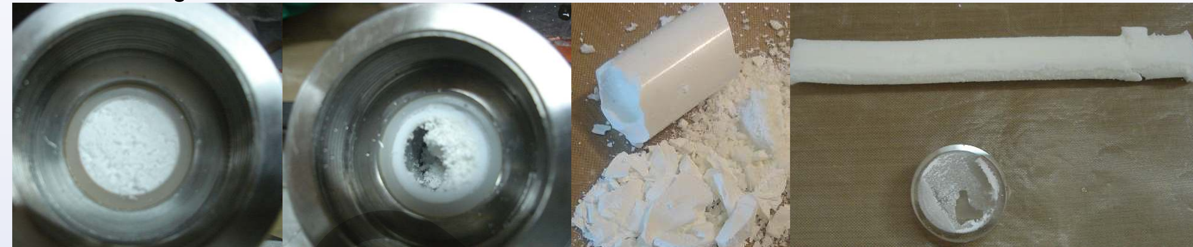
Cell full of PSDVB. Final product, not high monomer conversion. PSDVB with Krytox 257FSL as surfactant. PSDVB with PSDMS as surfactant.
