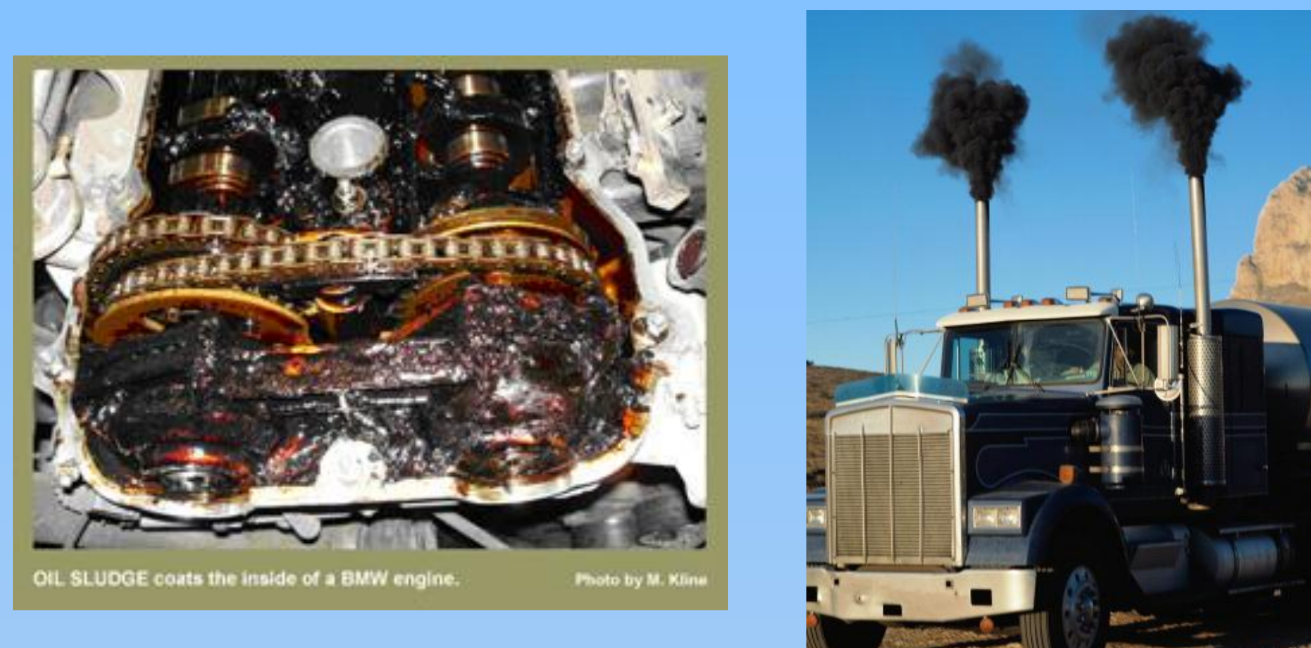
Figure 1: Sludge formed in the engine (left), and fine particle emission (right).
