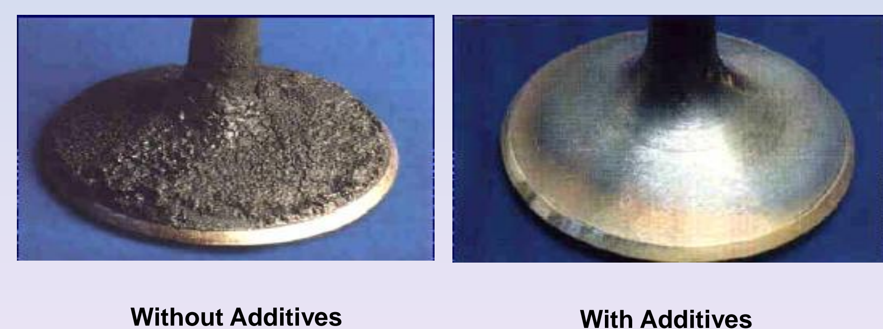
Figure 2: Two identical valves in a Mercedes engine after operating for 72 hours using engine oil with (right) and without (left) oil additives.
