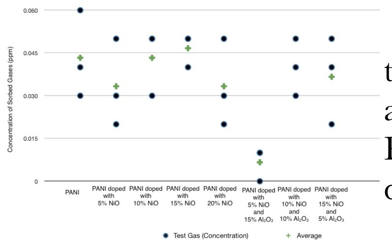
PANI and various doped PANI were tested for sensitivity towards formaldehyde at a concentration of 0.09 ppm (or 90 ppb). PANI doped with 5% NiO and 15% Al<sub>2</sub>O<sub>3</sub> did not detect at such a low concentration.
