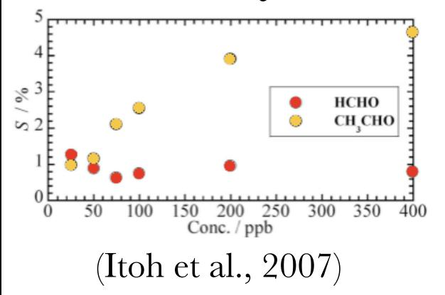
A sensitivity below 0.08 ppm is required for the detection of HCHO (WHO, 2001). The signal (S) is graphed versus concentration. The lower the concentration at which a signal is recorded, the more sensitive the sensor is.
