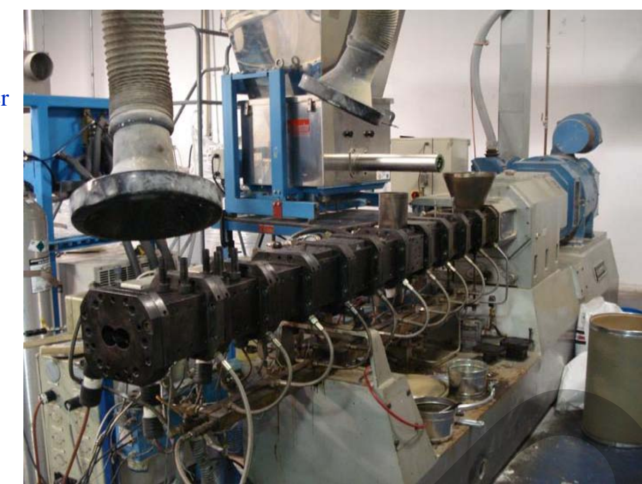
50 mm twin screw extruder (Leistritz Inc. Nj)
