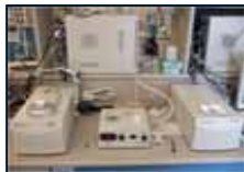
Fig 8. ITC Technique measures thermodynamic heat changes as a ligand is titrated into a titrant
