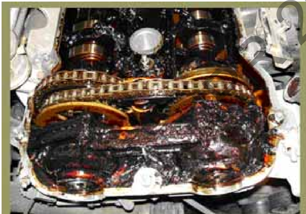
OIL SLUDGE coats the inside of a BMW engine.
