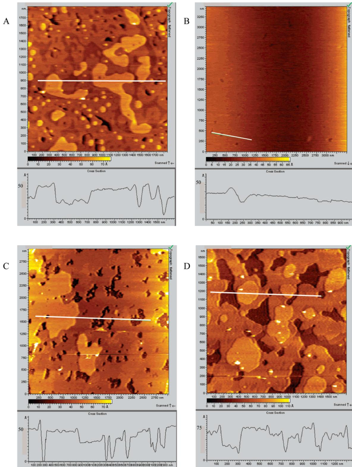
**Figure 1.** Heating a supported mixed DPTAP/DPPE bilayer, formed from an aqueous vesicle solution, 0.3 mg/mL, by pipetting 50  $\mu$ L; time of incubation on mica: 10 min. Key: (A) room temperature, 22  $^{\circ}$ C; (B) heated to 70  $^{\circ}$ C; (C) cooled back to room temperature, 23  $^{\circ}$ C; (D) cooling to room temperature after heating to 50  $^{\circ}$ C.
