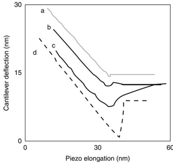
Fig. 2. Cantilever deflection  $dZ_c$  as a function of the piezotube elongation when the tip is retracted from the sample. DPPC bilayers deposited on mica were measured under three conditions: (b) the DPPC bilayer at  $T = 20^\circ\text{C}$  (c) the DPPC bilayer at  $T = 50^\circ\text{C}$  (d) the DPPC bilayer with halothane incorporated. The adhesion curve on bare mica (a) is shown for comparison.
