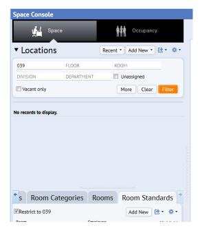
Underneath the list of drawings, you will find several tabs. These tabs will give you different slices of the data. However you also have to change the option for highlighting in the top band so it corresponds to the data you are looking at in the tabs. That way it will provide a legend for the colouring.
