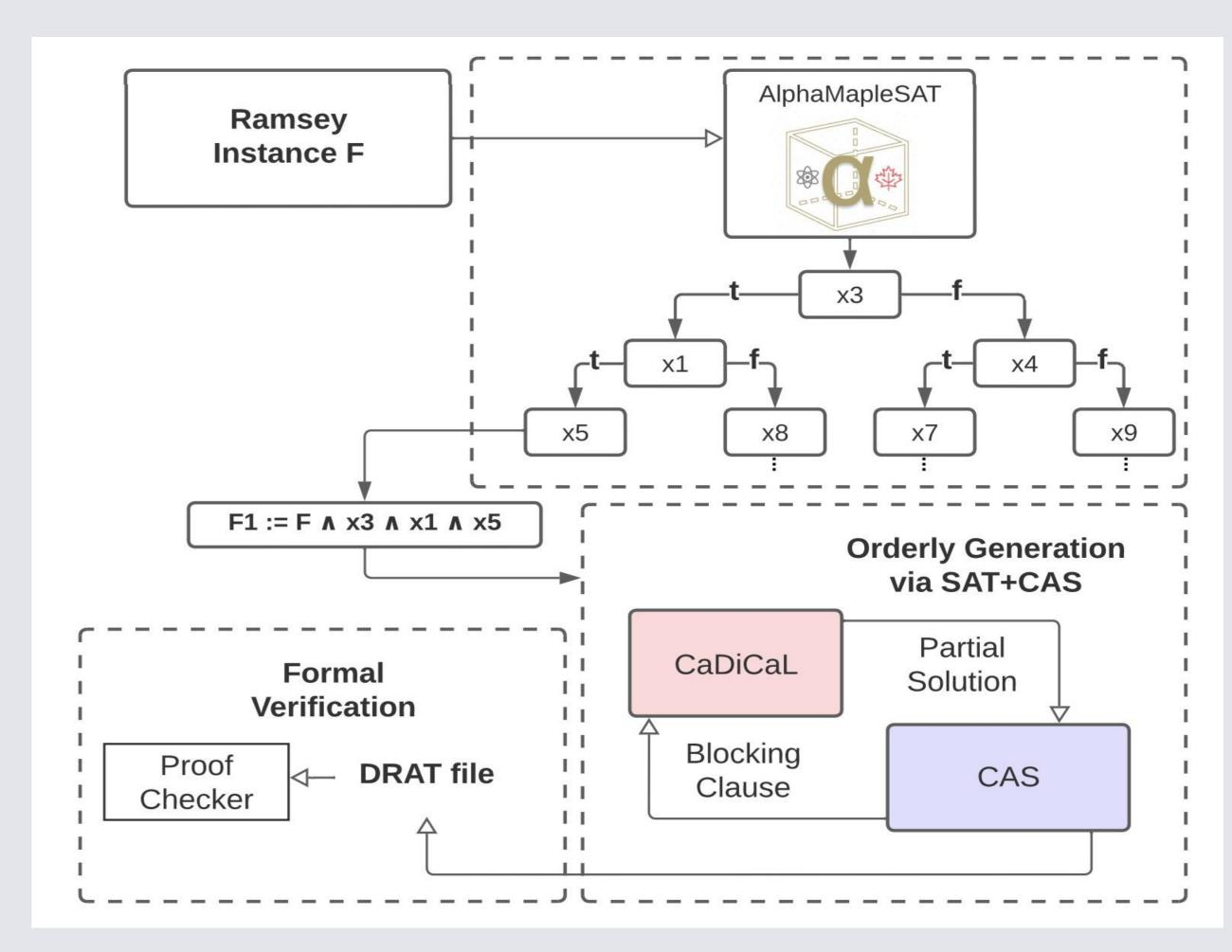
Flowchart of the parallelized MathCheck tool. AlphaMapleSAT is used as the cubing solver, and CaDiCaL + CAS is used as the conquering solver.
