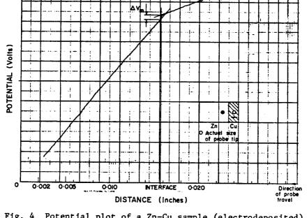
Fig. 4 Potential plot of a Zn-Cu sample (electrodeposited).
