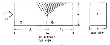
Fig. 6 Current flow through a sample.
