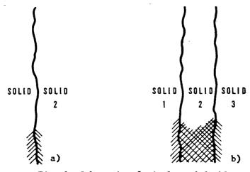
Fig. 1 Schematic of single and double continuous contact interfaces.
