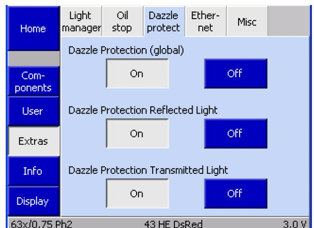
**Fig. 4-60** Page Microscope -> Settings -> Extras -> Dazzle protect
