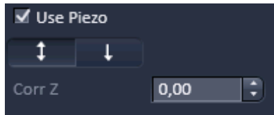
Fig. 79 Use Z-Piezo stage for Z-Stack acquisition – appearance for the LSM imaging mode
