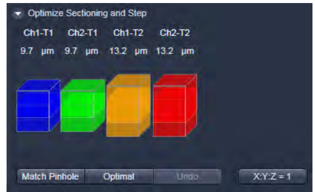
Fig. 80 Optimize Sectioning and Step: Optimal Interval is set starting with one Airy unit for all channels
