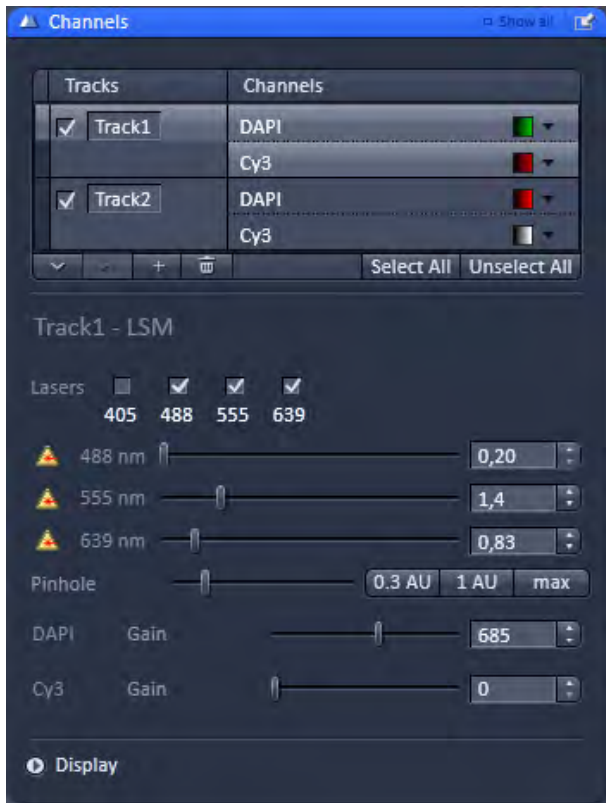
Fig. 72 Channels tool using channel mode (in this case multiple tracks) for imaging
