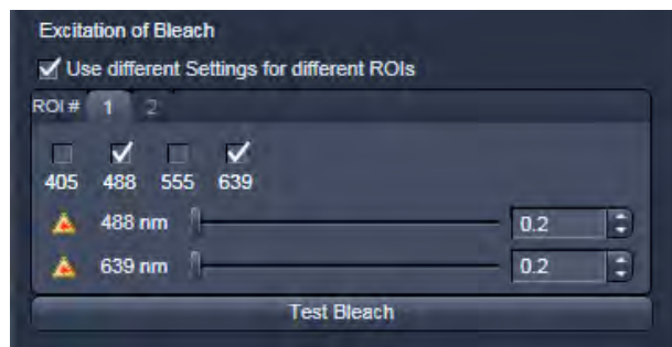
Fig. 85 Excitation of Bleach area for setting laser line and intensity for bleaching
