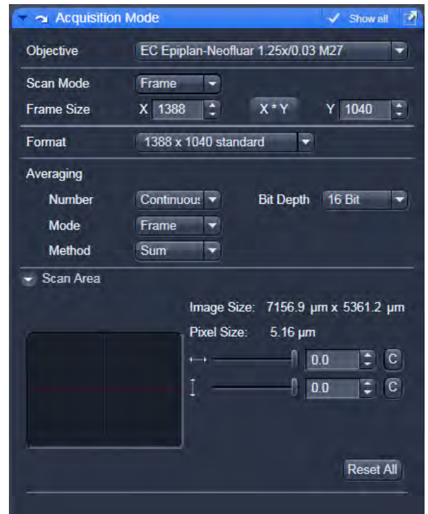
Fig. 69 Acquisition Mode - Frame with Camera tab selected in the Light Path tool
