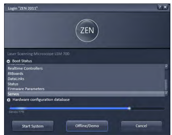
Fig. 8 Starting the ZEN software – The Login "ZEN" dialog with Boot Status field expanded and during the process of booting
