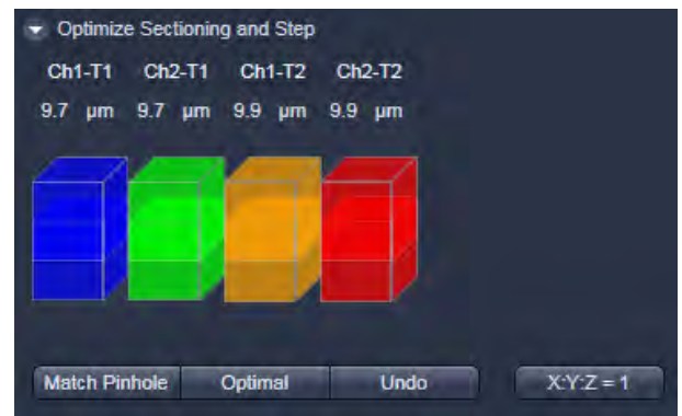
Fig. 81 Optimize Sectioning and Step: Match Pinhole to Step resulting in equal optical sections for all channels
