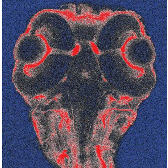
Fig. 103 Image displaying bad adjustment of gain and offset (blue regions are underexposed, red regions are overexposed)
