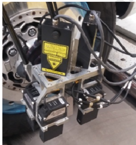
Fig. 3: LGS and LDV sensor set mounted on wheel hub
