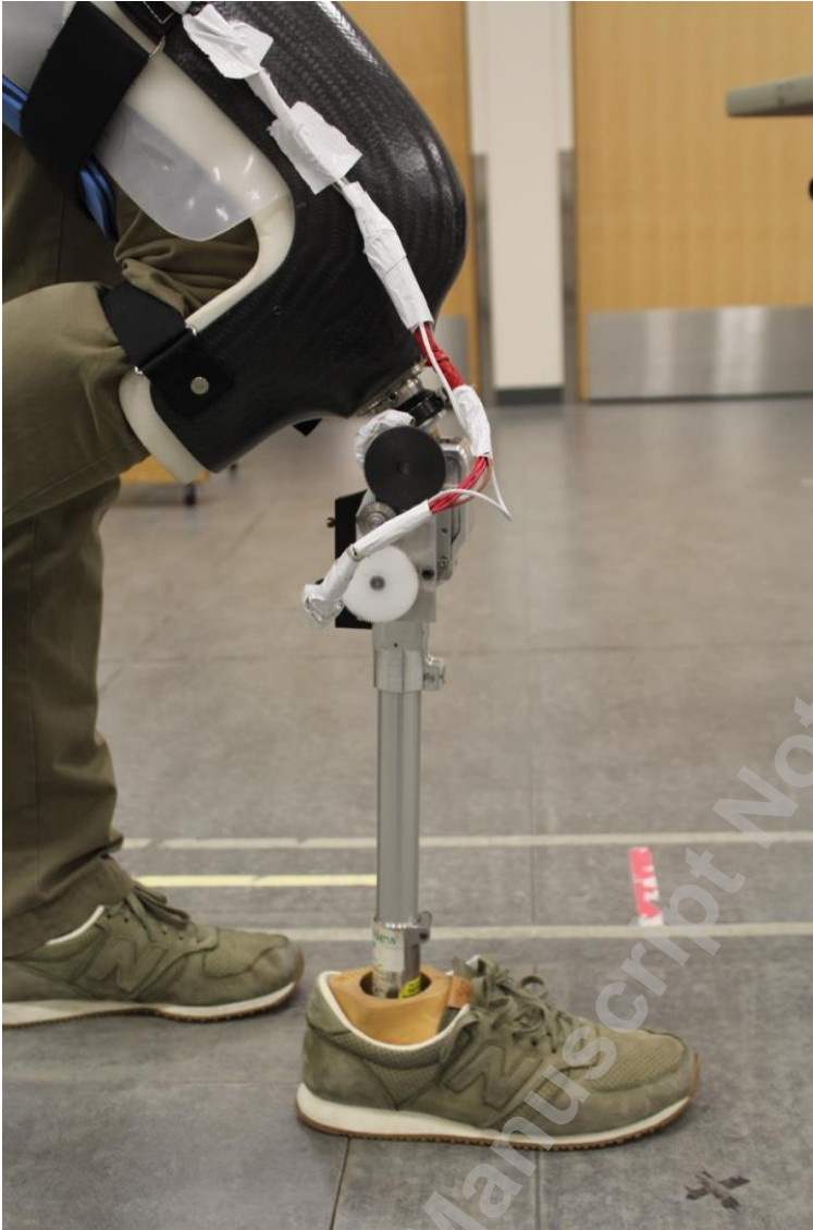
Fig. 3 Photograph of the regenerative braking semi-powered lower-limb prosthesis designed and prototyped by Dr. Jan Andrysek (University of Toronto, Canada)
