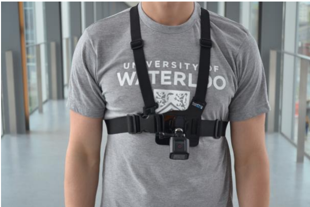
Fig. 3 Photograph of the wearable camera system used for experimental data collection and environment recognition.
