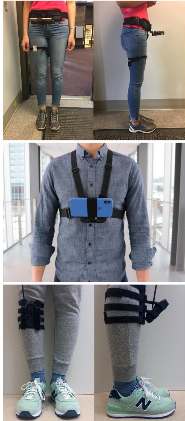
Fig 2. Examples of wearable camera systems used for environment sensing. The top and bottom photographs were provided by Dan Simon (Cleveland State University, USA) and Huseyin Atakan Varol (Nazarbayev University, Kazakhstan), respectively.
