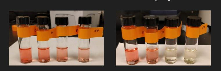
**Figure 7**: Decolourization of Allura Red AC with varying concentrations of HOBT. L to R: 0x HOBT, 1x HOBT, 5x HOBT and 15x HOBT.
