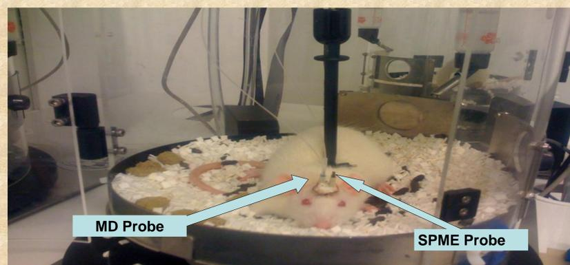
Figure 1 Simultaneous *in vivo* sampling from left and right brain hemispheres of a freely moving rat using microdialysis and SPME probes
