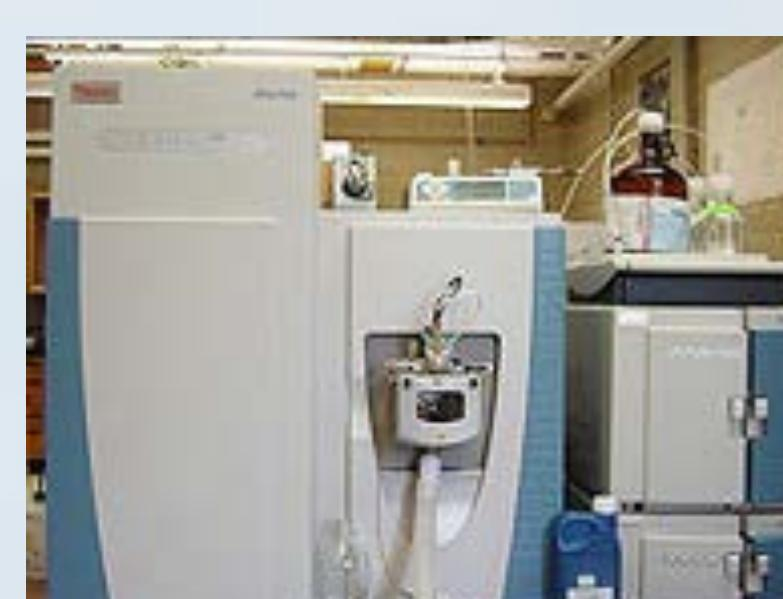
Exactive orbitrap mass spectrometer operated in positive and negative mode
